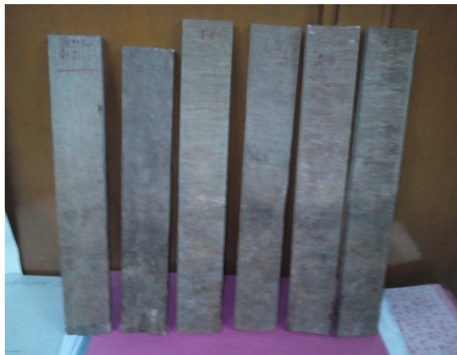
Fig 2 : Samples after exposure to termite test
